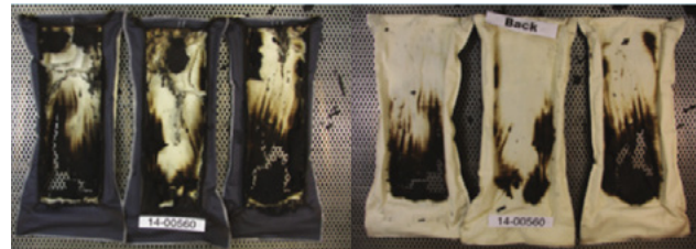
Front- exposed to arc flash
