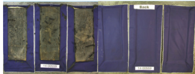
Front- exposed to arc flash
